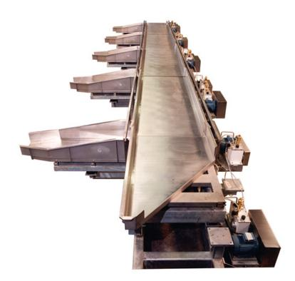
The Distribution Conveyor System allows processors to increase production and efficiency by feeding multiple processes from one system. Its vibratory conveyor moves product to feed each discharge point, with optional pneumatic gates ensuring standard flow to each with no starvation. Its stainless steel construction and solid pans allow for quick, yet thorough cleaning.
