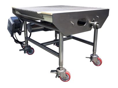
The Spreader links the key processes of your line by spreading, diverging, or converging product between wider and more narrow belts. Its positive drive, non-slip stainless steel flex wire chains position product seamlessly, with no jams or pile ups. Tight infeed and outfeed transfers ensure product orientation and integrity. The Spreader is designed for easy sanitation and maintenance.
